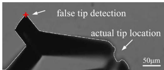
Fig. 9. Autolocating microgripper tips failed due to other structures appeared in the FOV first.
