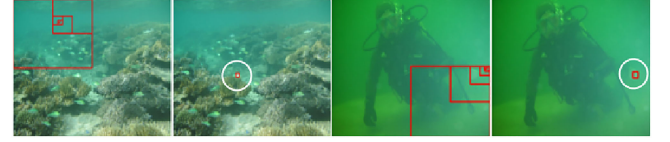
Fig. 4. Quad-tree subdivision to get the highest-intensity region of the underwater image for B_c estimation.
